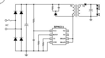
Figure 1. Typical application circuit for BP9021A
